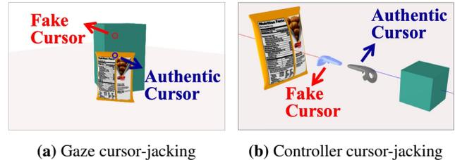
**Figure 2: Illustration of (a) gaze and (b) controller cursor-jacking attacks: (a) When a user clicks a UI button via the gaze cursor made by the attacker, the authentic cursor clicks the ad. (b) Inserting a fake controller cursor by rotating its z-axis by 180 degrees. When a user clicks the green box with an authentic VR controller cursor, the ad placed in the opposite direction is also clicked.**
